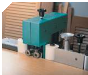
Power trimming unit: Trimming strip on both sides simultaneously.
