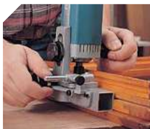
Slotting a window, flashing side.
