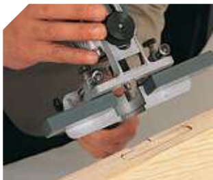
Placing hinges with the ZB93 head.
