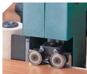
Power trimming unit: trimming both sides simultaneously.
