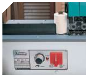
Electronic temperature regulation.
