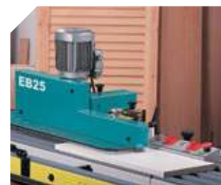
Feed unit: feeding of the workpiece to be edged.
