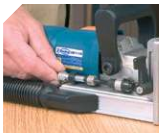
Quick adjustment of different slotting depths.
