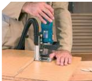
Joints in middle of board.
