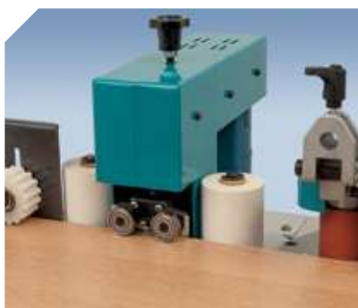
Trimming unit for tapes up to 1 mm thickness.
