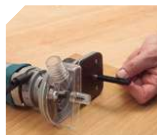
Precise guiding for corner trimming.
