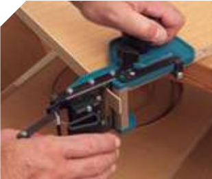
Cutting on both sides on straight panels.
