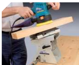
Folding and rotary adjustable support.
