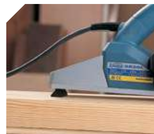
Rest shoe to avoid the blades touching and damage the surfaces.
