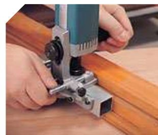
Slotting a window, lock side.
