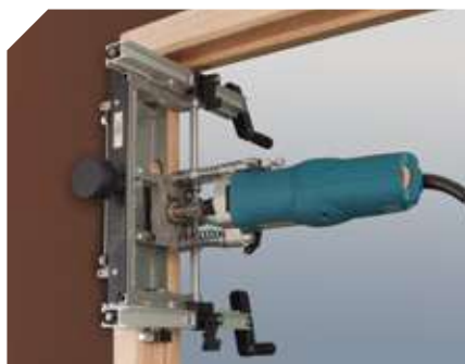
Making the upper recess on the frame.
