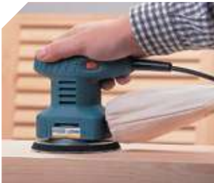
Like rotary orbital it combines two movements: rotary and orbital.
