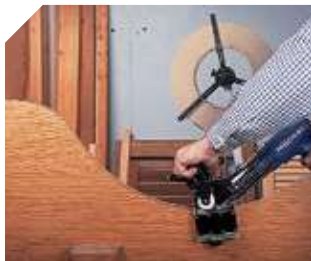
Enables banding of circular or shaped pieces.
