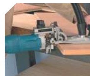
Trimming the edge with the straight bit.
