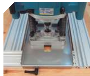
The use of PF400 and PF700 templates allows multiple applications.
