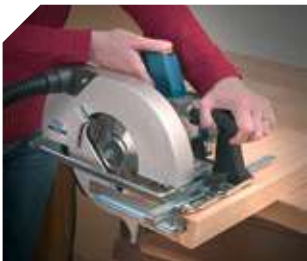
Performs cuts of up to 70 mm.
