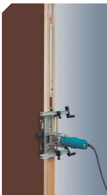
Making the second recess on the frame.
