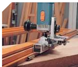
Slotting a window, hinges side.
