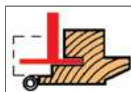
Slotting a window, hinges side.
