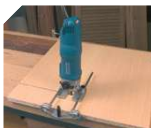
Trimming parallel slots.
