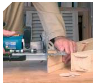
Stronger joints with No. 6 splines.
