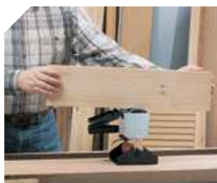
Gluing with the upper roller.
