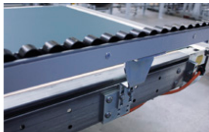
Small roller gib to support wide workpieces (option)
