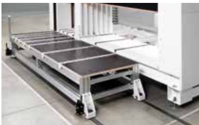
Sliding pre-plugging station: The pre-plugging station allows a simple assembly of the carcasses at working height of the press.
