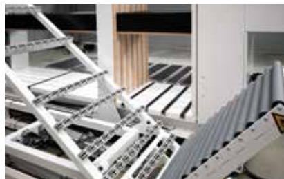
Manual cabinet uprighter: The cabinet uprighter is used for the uprighting and onward transport of assembled cabinets.
