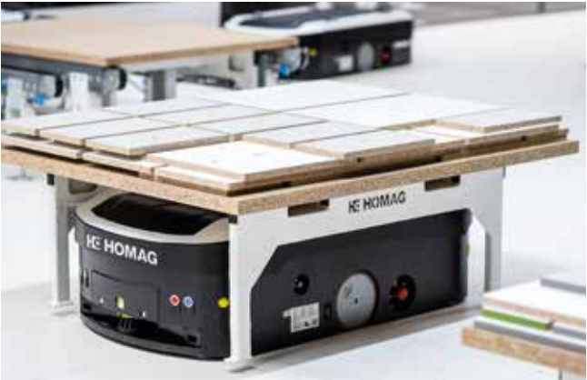
Automated guided vehicle system TRANSBOT S-100. TRANSBOTs arrange the material transport between stacking and feeding station. It transports a maximum weight of 1.2 tons at a travel speed of up to 60 meters per minute.
