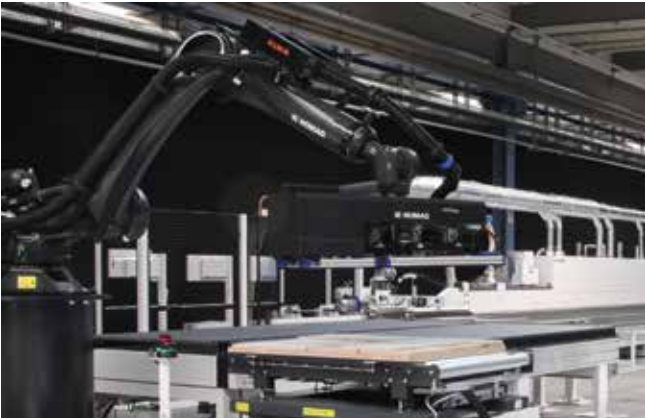
Feeding robot FEEDBOT E-300. With the assistance of camera technology from KUKA, the robot recognizes every workpiece in the stack and places it precisely, with an availability of close to 100%, in the feeder station of the edge banding machine.
