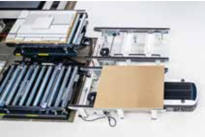
The transfer station with lift table raises a material stack until the top layer reaches the ideal height for the FEEDBOT.
