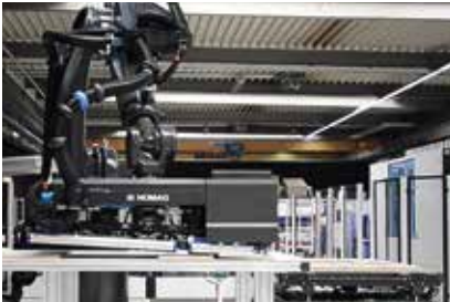
Workpieces are temporarily stored in the sorting station at the entry to the edge banding machine until they fit perfectly into the stacking pattern that is formed by the stacking robot after a process run.
