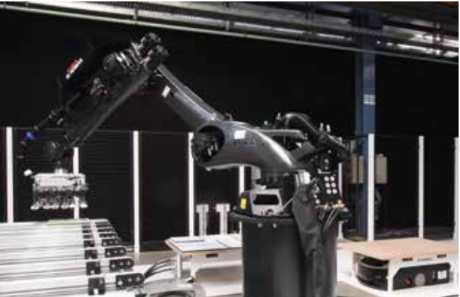
Stacking robot STACKBOT E-600. Workpieces coming out of the edge banding process are picked up from the exit conveyor by the robot and placed precisely at the intended position on the stack.
