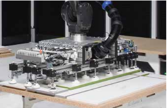
Intelligently sorted stack formation for high stability. After every process run the material stacks are formed intelligently so that as many parts as possible are in one layer.
